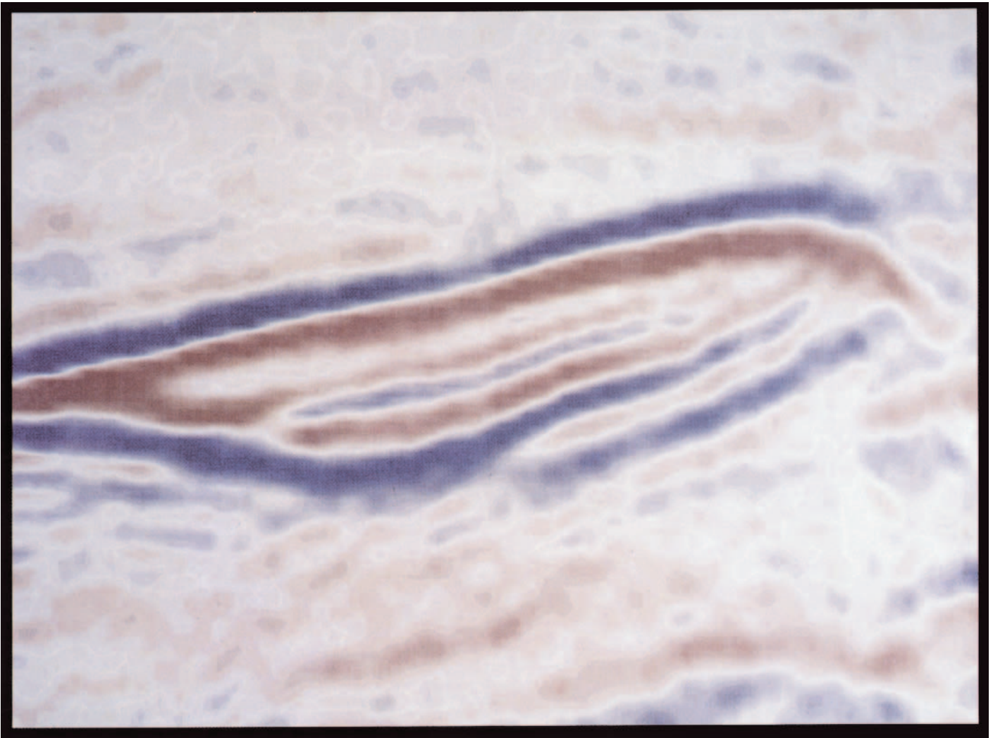
Fig. 2-27. Gulf of Mexico shallow gas reflections showing a phase of approximately 90^\circ . (Courtesy Mobil Exploration & Producing U.S. Inc.)
