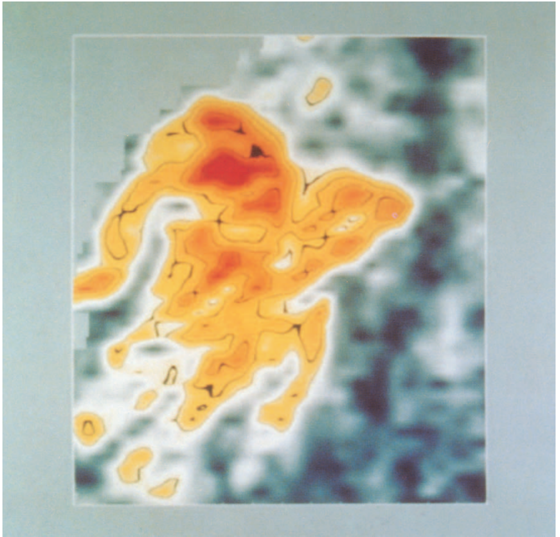
Fig. 2-33. Same horizon slice as in Figure 2-31 displayed in reds, yellows and grays to accentuate total drilling potential. (Courtesy Chevron U.S.A. Inc.)
