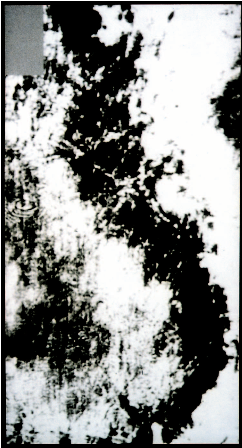
Fig. 3-43. Horizontal section at 646 ms from high resolution 3-D survey at Ekofisk field in the North Sea. Note lineations due to faulting and jointing. (Courtesy Phillips Petroleum Company Norway.)
